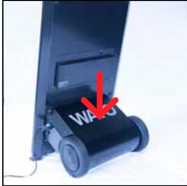
WAYO's battery can be charged by connecting the charging cable to the device then plugging the other end into a power point.
