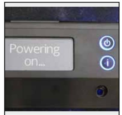
To turn off your WAYO, hold the power button for three seconds.
