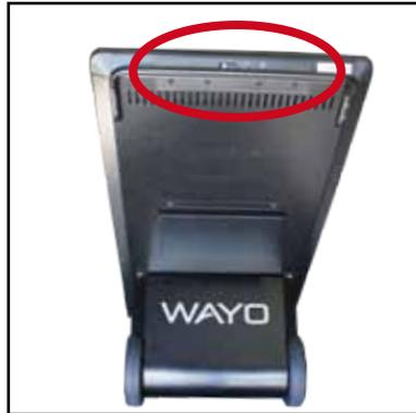
The control panel is where you turn your WAYO on and off, and where you can read the battery life status and its serial number.
