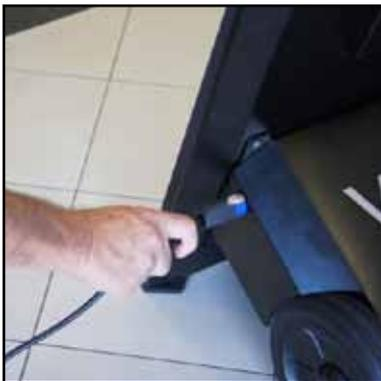
Once your WAYO has been charged, remove the power cable by sliding the thumb lock on top of the connector plug back away from the device
