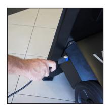
Once your WAYO has been charged, remove the power cable by sliding the thumb lock on top of the connector plug back away from the device
