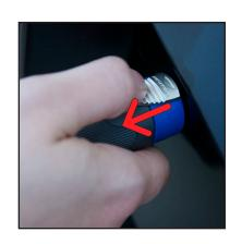
Twist the connector plug anti-clockwise one quarter of a turn and carefully pull it out.
