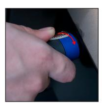
Check to ensure that the cable is securely connected and that the device is charging.
