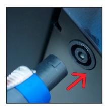
Push the connector in, and twist clockwise one quarter of a turn to lock the connector in place.
