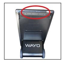
The control panel is where you turn your WAYO on and off, and where you can read the battery life status and its serial number.
