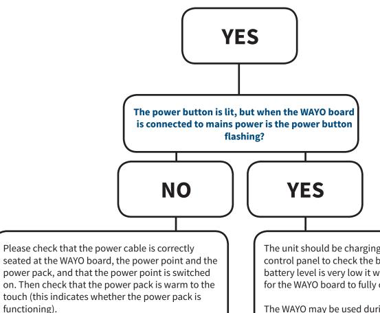
If the cables are correctly seated and the power point is switched on and the power pack is warm to the touch, please contact WAYO support.
